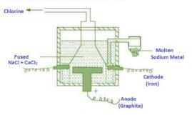
A graphite block is the anode while steel is made the cathode. Metallic Ca and Na are formed at the cathode Molten Na is supported by dipping in kerosene.
