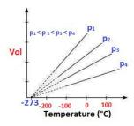
It was found that for all gasses (at any given pressure), the plot of volume vs. temp. (in °C) is a straight line.
